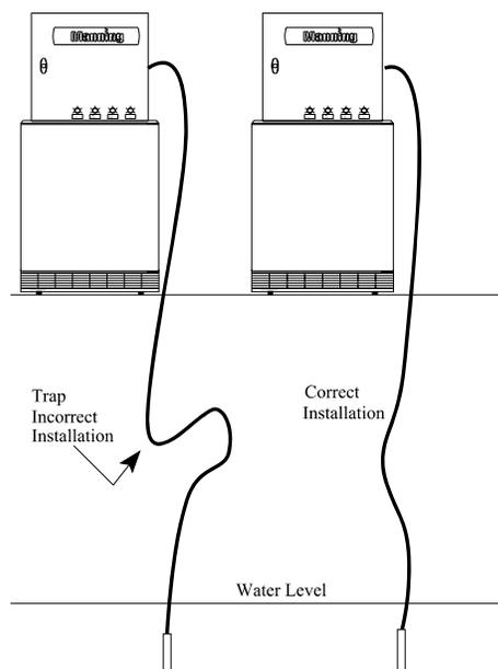
Figure 1-13 Intake Hose Placement
