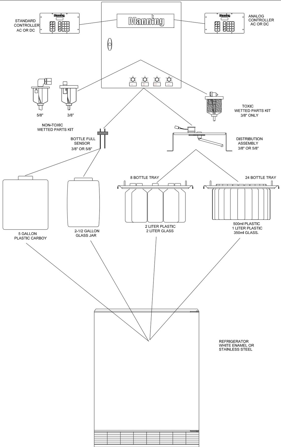
**Figure 1-1 6901 Stationary Sampler Components and Assembly**
