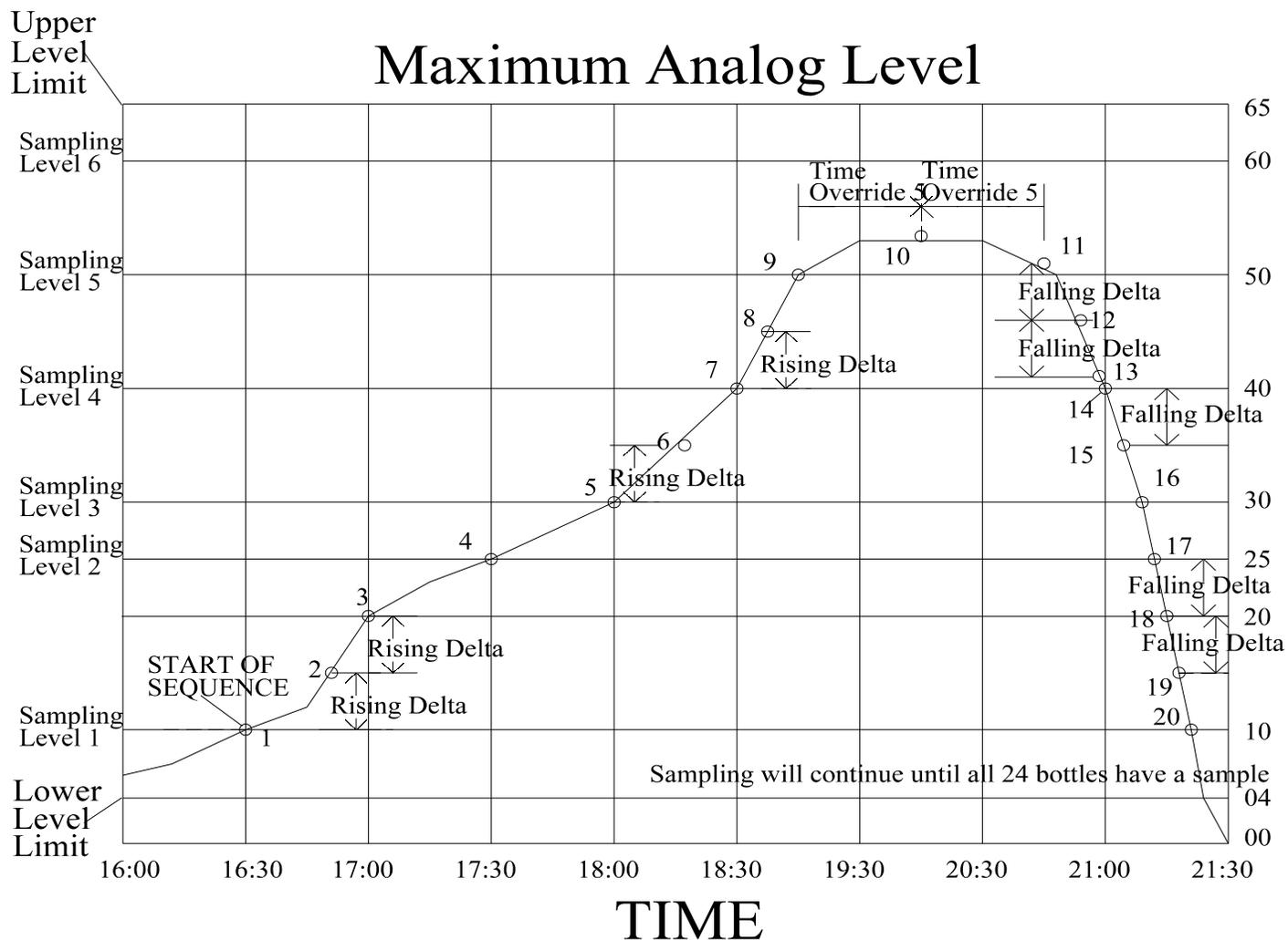
**Figure 2-3 The \*09 Storm Water Sampling Mode**
