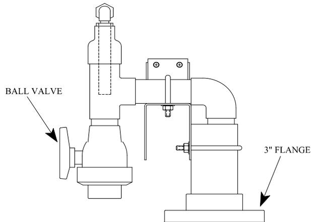
**Figure 1-3 The Flow-thru Cell (older version- mounts to side of sampler)**
