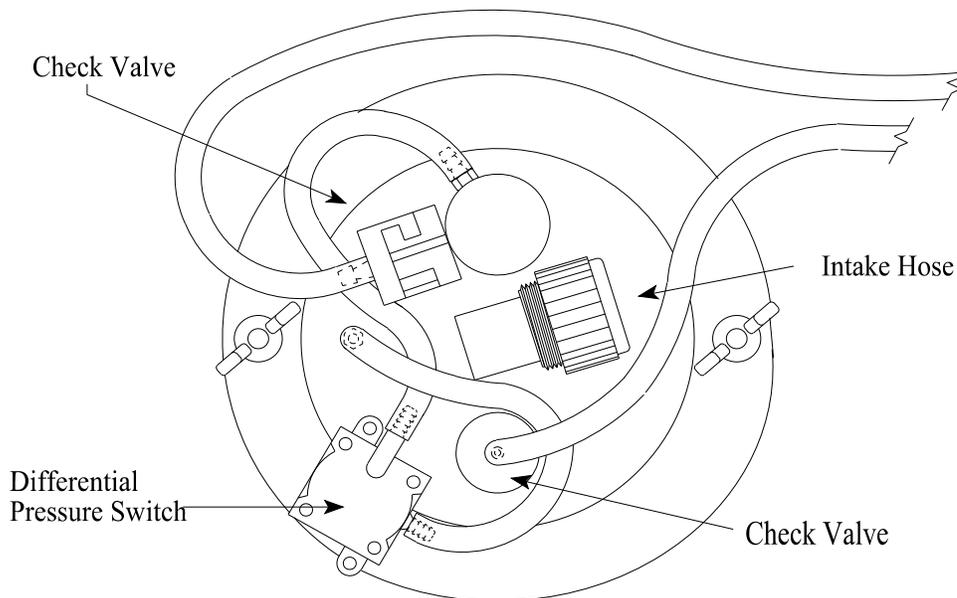
**Figure 1-12 Insertion of Intake Hose into Chamber Top - Priority Pollutant Option**
